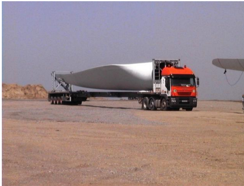
Delivery of GE “oversized components” (blades)
